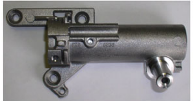
Figure 5: Thixoforming cell at Madison-Kipp Corp. and SiBloy® SSM castings produced.
