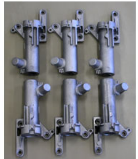
Figure 5: Thixoforming cell at Madison-Kipp Corp. and SiBloy® SSM castings produced.
