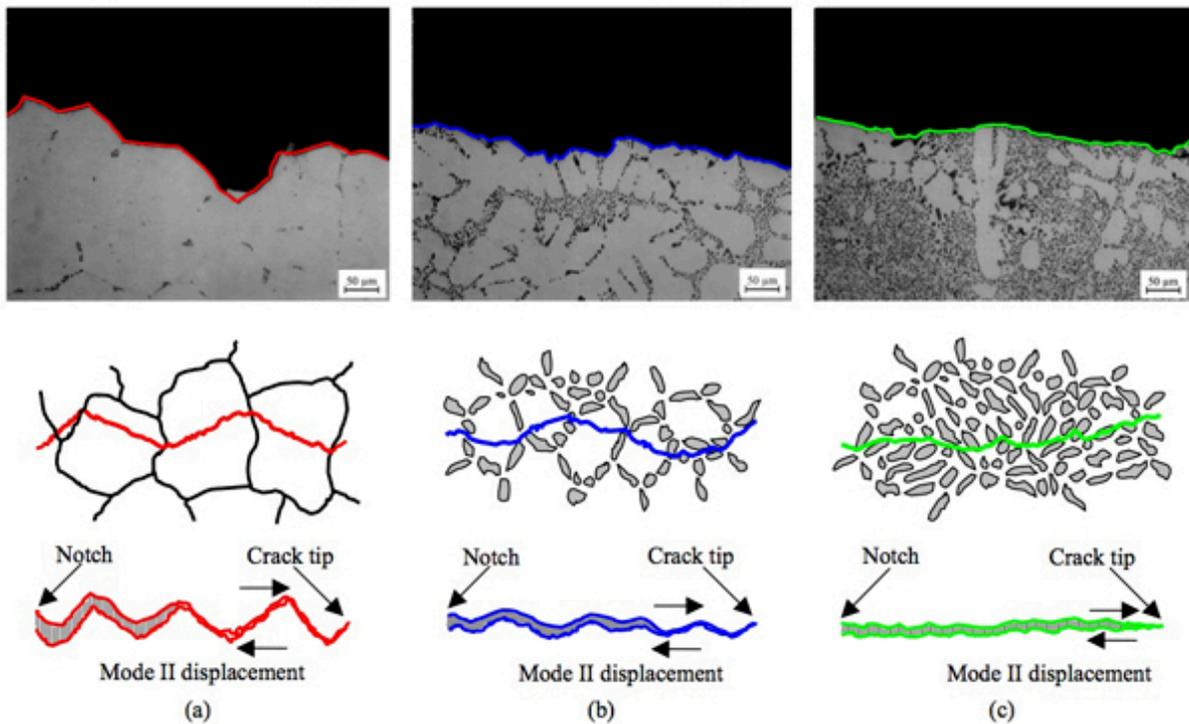
Figure 4. Crack path deflection patterns for three Al-Si-Mg alloys: (a) 1%Si; (b) 7%Si; (c) 13%Si (fractographic observations - top and crack path models - bottom); mode II displacement is also contributing to closure.
