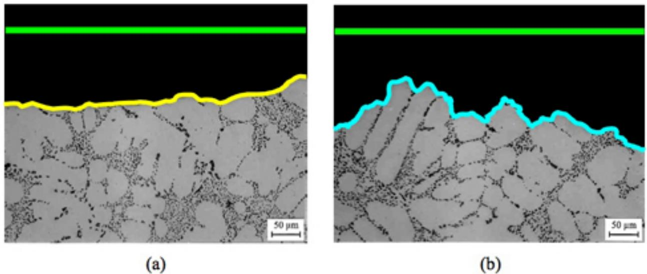
Figure 5. Changes in fracture surface roughness with increasing crack driving force for a Sr-modified 7%Si alloy: (a) lower Region II ( $\Delta K \sim 5.5 \text{ MPa}\sqrt{\text{m}}$ ) and (b) lower Region III ( $\Delta K \sim 12 \text{ MPa}\sqrt{\text{m}}$ ).
