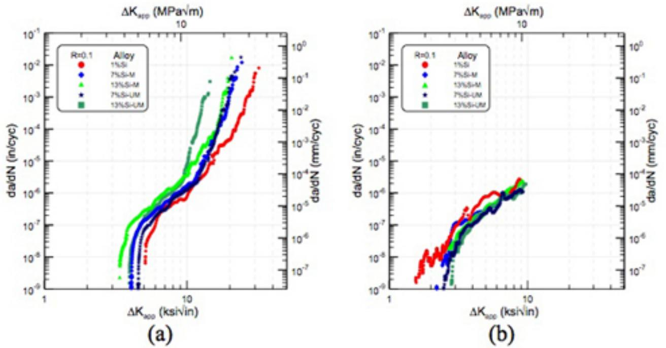
Figure 3. Fatigue crack growth data for 1, 7, and 13%Si cast Al-Si-Mg alloys with low residual stress: (a) long crack growth data and (b) small crack growth data.
