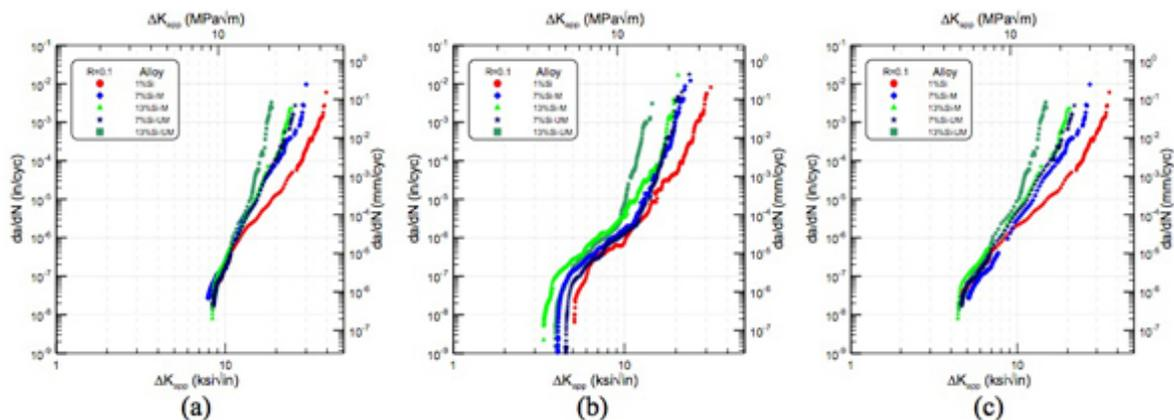
Figure 2. Fatigue crack growth behavior of the five studied alloys in high residual stress conditions (a), low residual stress conditions (b), and high residual stress conditions after residual stress correction (c).
