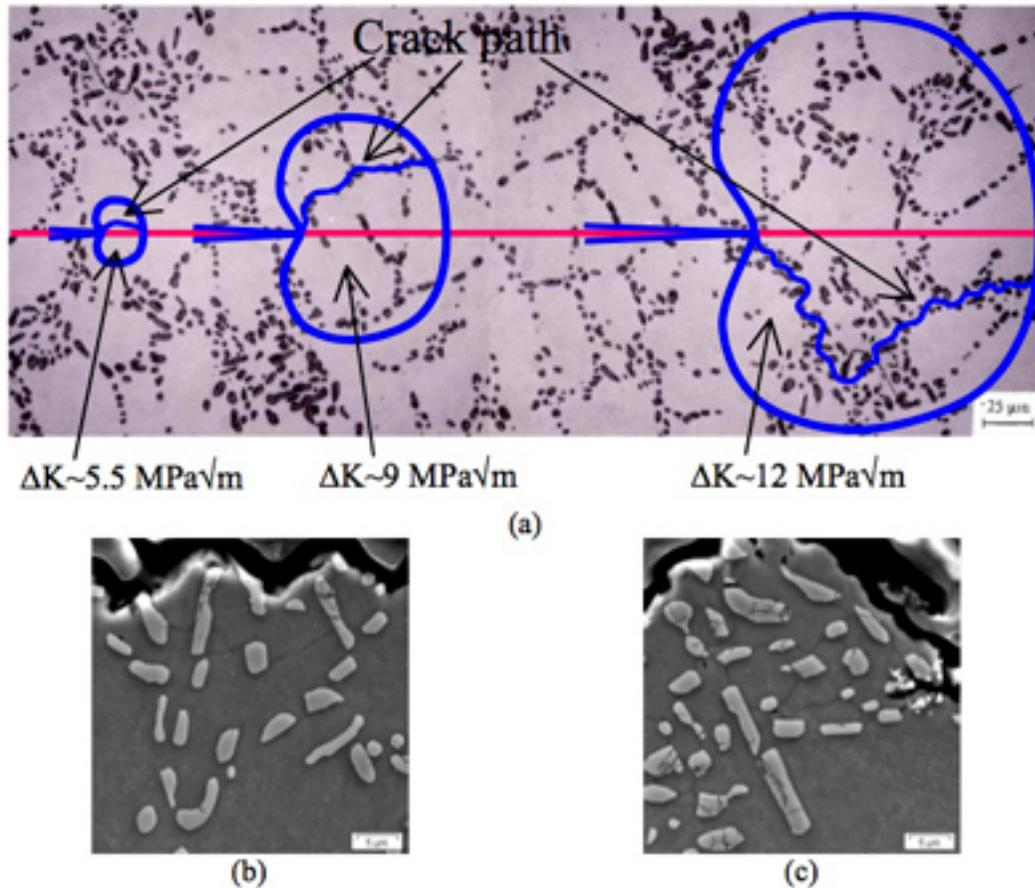
Figure 6. (a) Plastic zone size representation at the microstructural scale of a 7%Si alloy for different  $\Delta K$  levels; enlargements of the damaged regions in the plastic zones at (b)  $\Delta K \sim 9 \text{ MPa}\sqrt{\text{m}}$  and (c)  $\Delta K \sim 12 \text{ MPa}\sqrt{\text{m}}$ .
