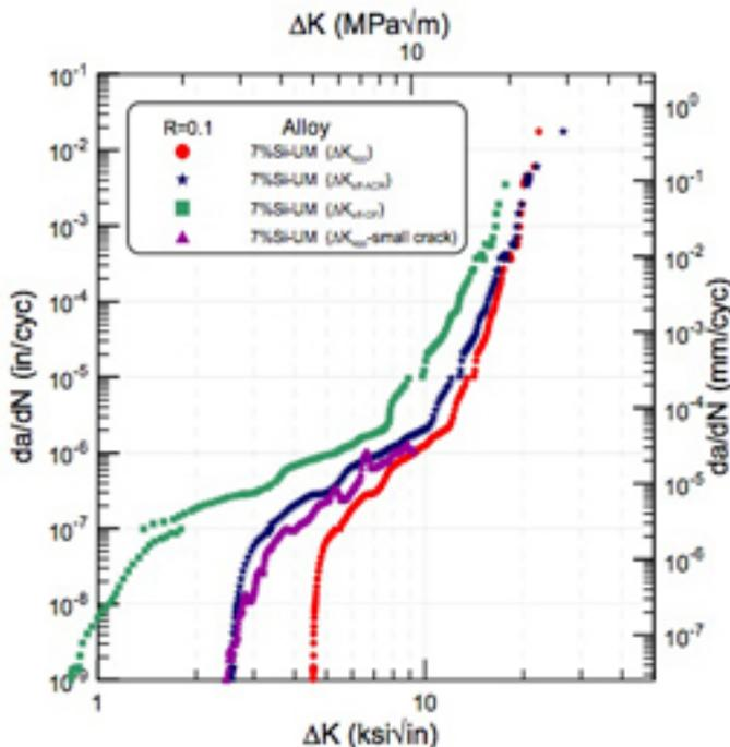
Figure 7. Comparison of long crack data, small crack data, and closure corrected data for an unmodified Al-Si-Mg cast alloy with 7%Si.
