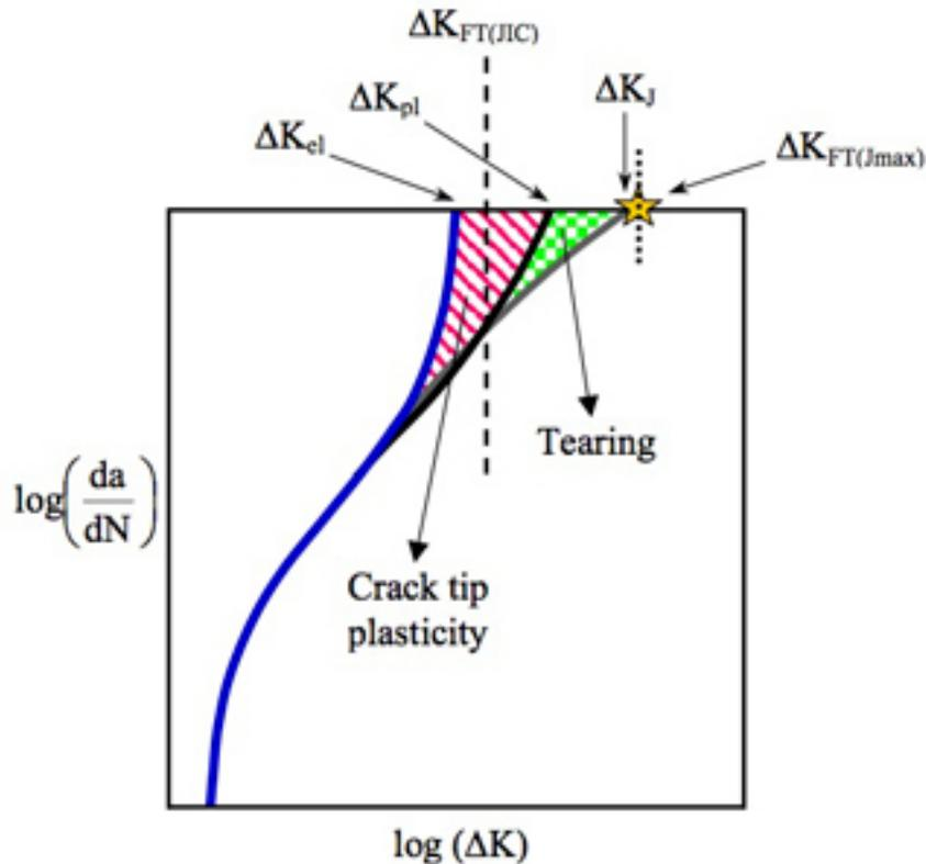
Figure 8. Enlargement of upper Region II and Region III showing the effects of plasticity and tearing and their respective interactions.
