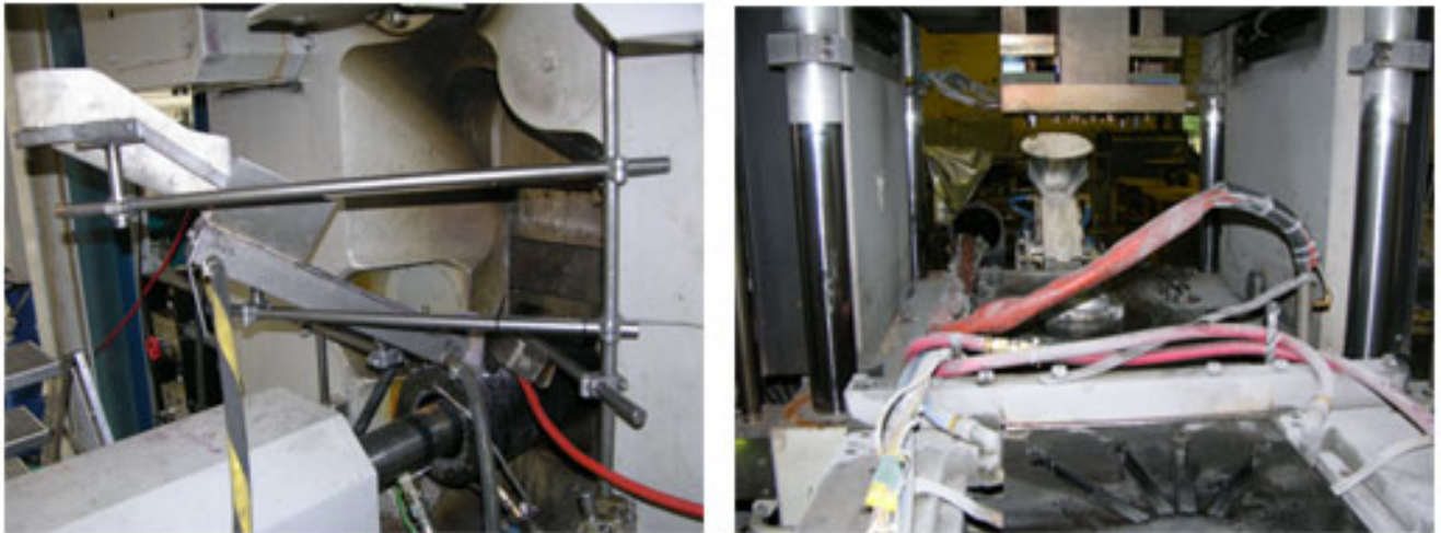
Figure 2: Showing the CRP reactor attached to a horizontal die casting machine (a), and a vertical die casting machine (b).
