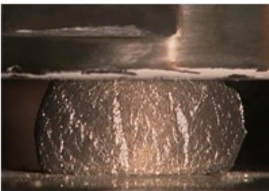
Figure 5: Flow behavior of A356 sample at different shear strains (temperature: 585°C; shear rate: 5.0 \times 10^{-3} \text{s}^{-1} ) (a) 0, (b) 31.9. The figures on the left are the experimental data and those on the right are the corresponding simulation results.
