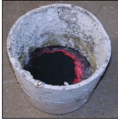
(2) plunging the mixture, which was previously encapsulated in aluminum foil, into the melt, or
